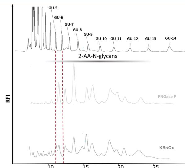
**Fig. 4:** Synoptic view of HILIC-FLD profiles of anthranilate labelled N-glycans from chicken ovalbumin. The pattern of ovalbumin N-glycans released by PNGase F matches the pattern released by Oxone® and bromide.
